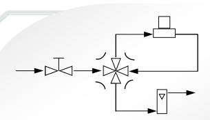
Integral bypass sample system significantly increases user productivity. The bypass valve isolates the sensor from high oxygen levels when changing sample lines. Maintaining low PPM oxygen levels allows the user to move from point to point without waiting.
